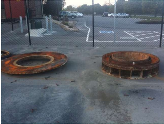
Original base and turntable, Biotower No. 1
